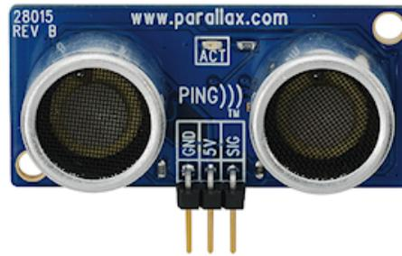
Figure 3.16: The Parallax PING))) Ultrasonic rangefinder used to detect small obstacles and objects in areas not visible to the LiDAR.
