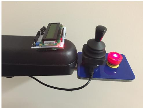
Figure A.6: Emergency stop, LCD indicator, and secondary joystick (for show only).
