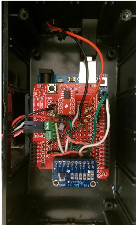
Figure 4.6: Constructed DAQ system. Not pictured: current sensor
