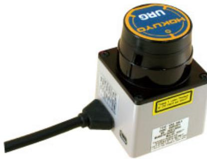
Figure 3.14: The Hokoyu URF-04LX LiDAR module used to map the environment around the wheelchair.
