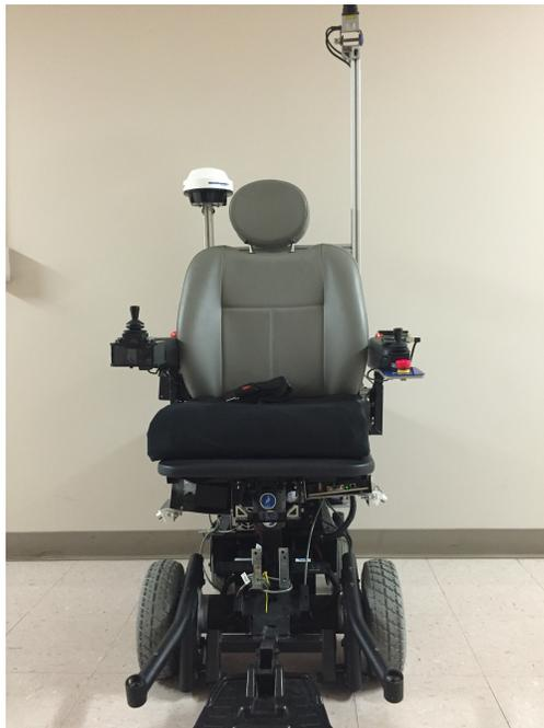
Figure A.3: Front-on view of the wheelchair
