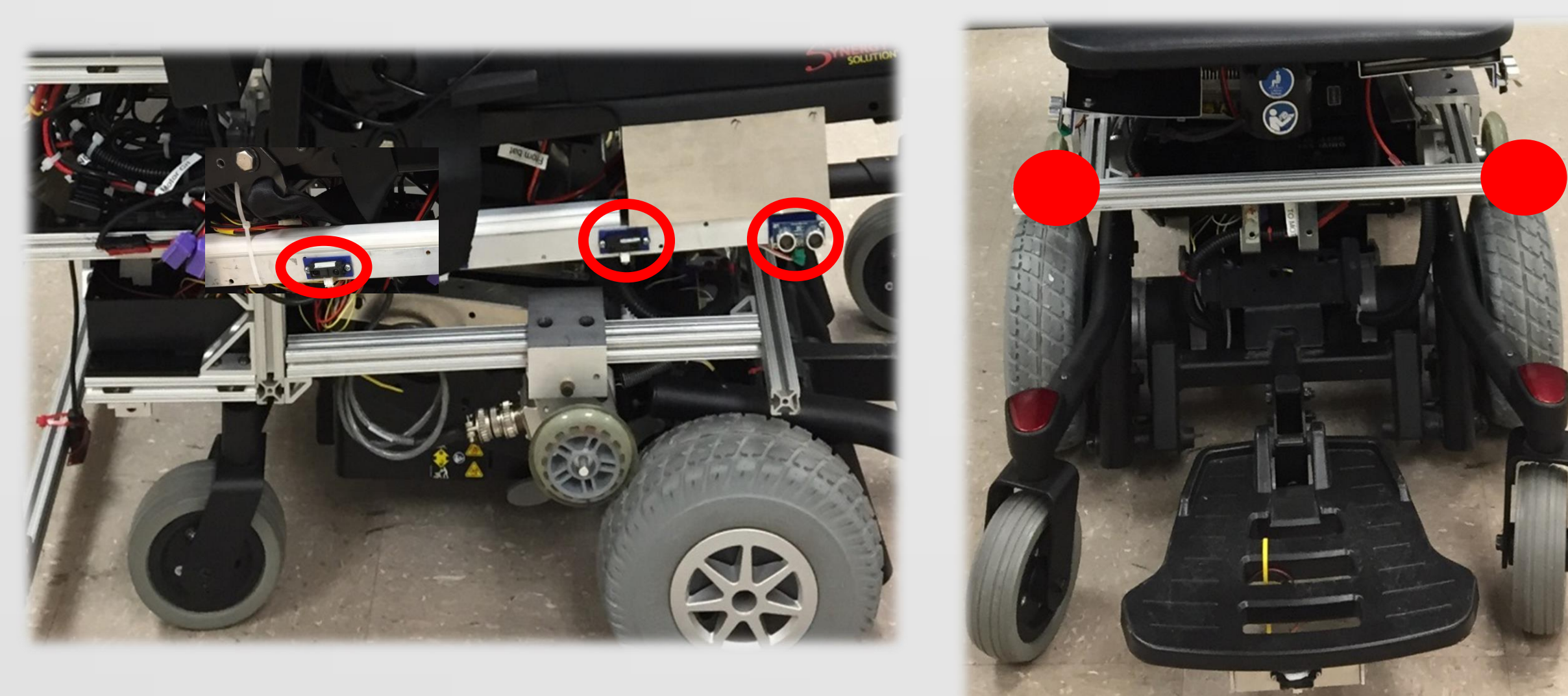
Sensors for drop off detection and small obstacle avoidance
