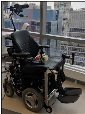
Fig 1: The custom autonomous wheelchair is composed of a Permobil C300 wheelchair, a computer running the Robotic Operating System (ROS), 23 two ASUS Xtion RGB-D cameras, 24 and a variety of control interfaces (joystick, head array, and sip-and-puff device).
